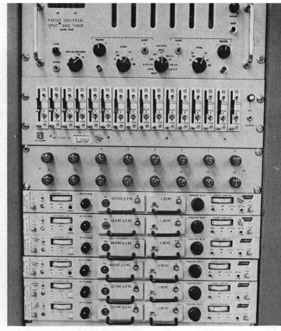
SPECIFIC TIME of events in shock tests are located by the IRIG timer and fed into this Present Universal Timer in Area III which measures event duration with microsecond accuracy.
